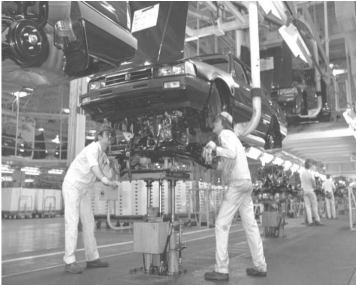
Marysville, Ohio, Honda factory workers install an engine on a 1983 Accord sometime in late 1982.
